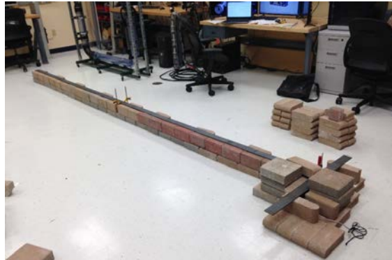
Fig. 10. Laboratory scale test bed created for determining the pull force created by tether.
