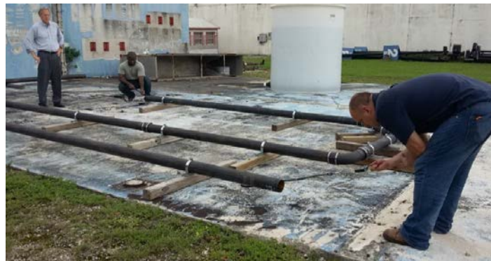
Fig. 20. Preliminary tether pull and drag testing.
